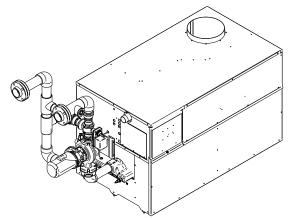
Figure 45 – Horizontal Pool Heater Piping
